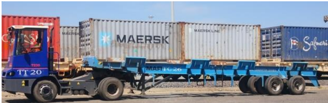
Figure 8 Existing tractor-trailer unit used at the Modjo Container Terminal
