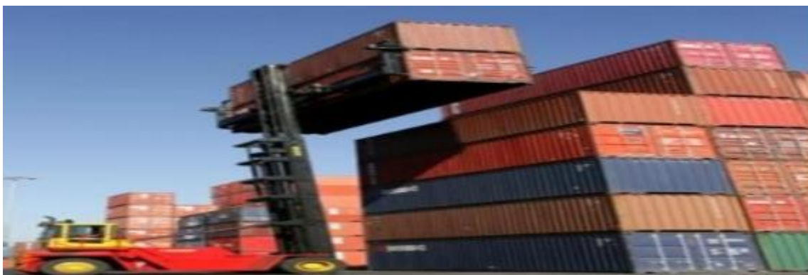
Figure 6 Empty Container handler
