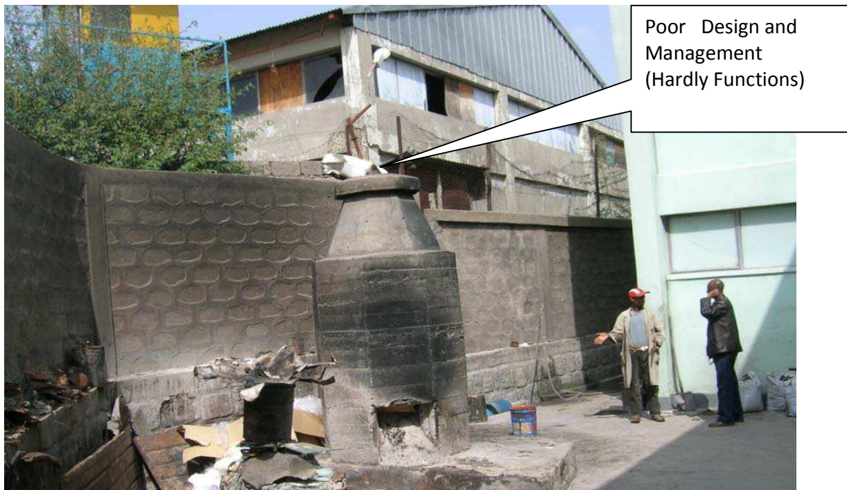
Fig. 3.5. Incineration on Site by MAMCO Paper Products Company (Observation of the researcher)
