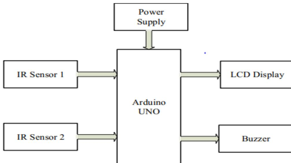
*Figure 2.7 Block Diagram of the speed detection System [23]*
