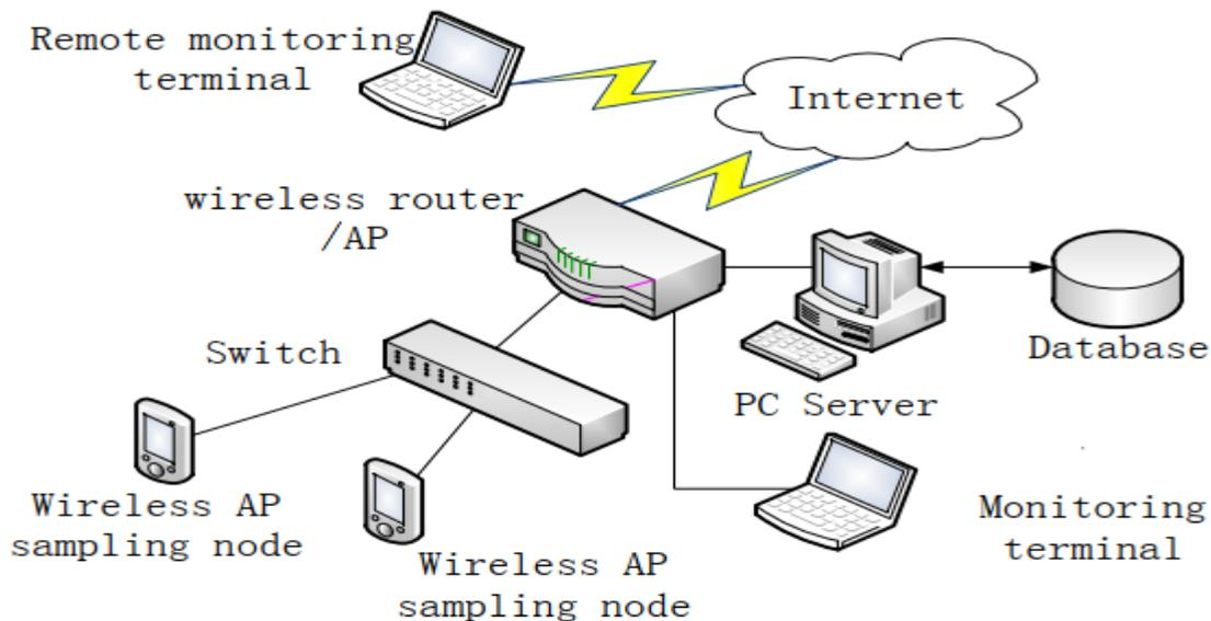
Figure 2.1, System architecture vehicle overload detection system [10]
