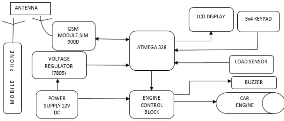
Figure 2.8 Block Diagram of the Vehicle Load Monitoring System with an automatic Engine Lock System based on GSM [24].
