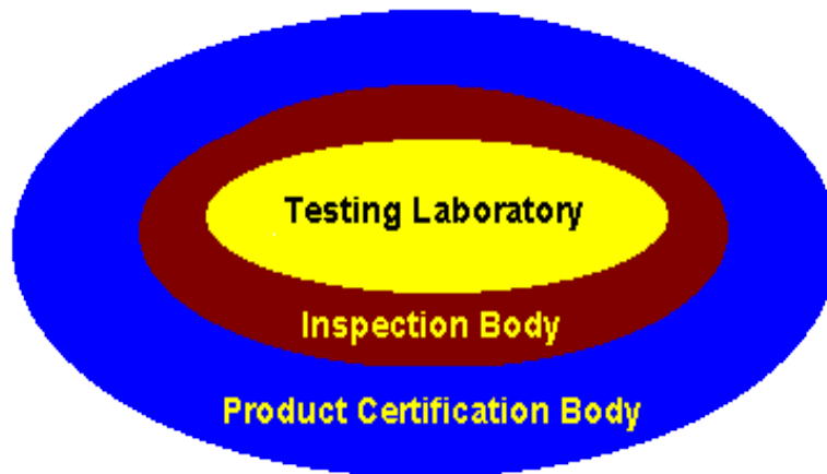
Figure 1. Model demonstrating the overlapping activities of the three bodies in relation to the determination of conformity with the requirements
