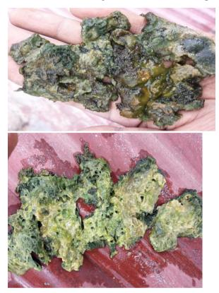
Figure: 4. 5 Algae Formed in Un-Cleaned Drinking Water Storage Tanks
