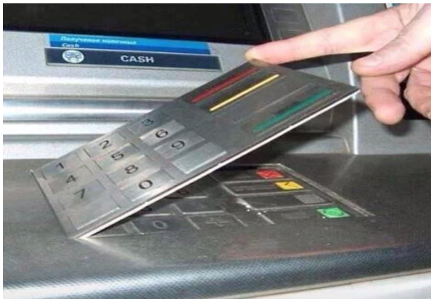
Figure: 2.4 Credit-card-skimming-explainer (Engadget)
